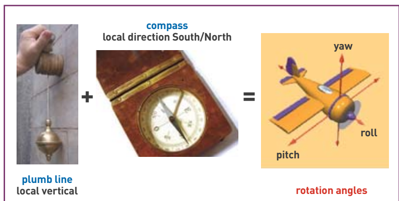
Figure 1. Method for evaluating rotation angles in a three-dimensional reference system, based on measurements of verticality and rotation in relation to magnetic north.
