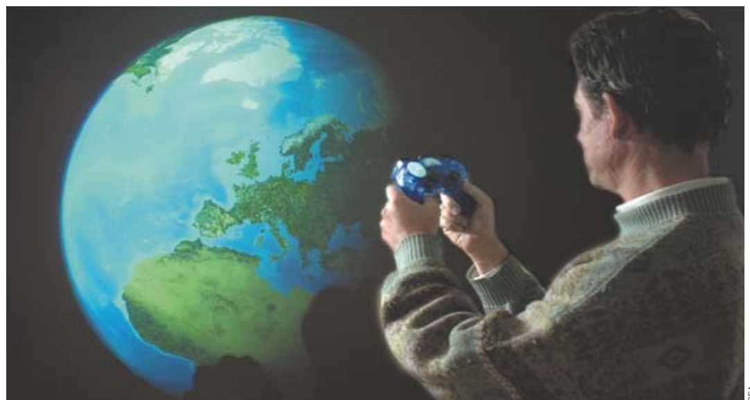
Interface with a 3D IGN database. Its navigational function follows the handle's spatial orientation.
